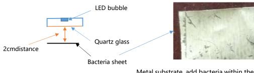
Metal substrate, add bacteria within the diameter of 1cm, the number of bacteria is  $5 \times 105 \sim 5 \times 106$ CFU, and the bacteria sheet is placed in the position where the UV lamp module is facing at.
