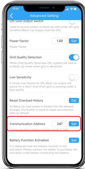
→Address must be set up on each inverter separately
