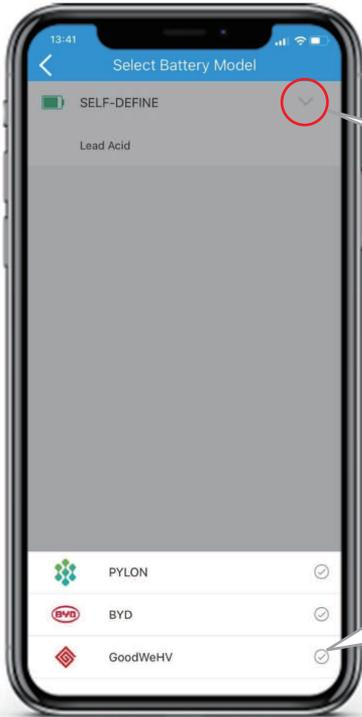
PV Master will read inverter information and selectively shows the compatible battery list.
