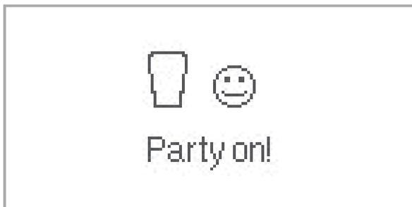
With the party function the storage temperature is heated up once to the reference temperature (Tref off), disregarding the set thermostat times.
