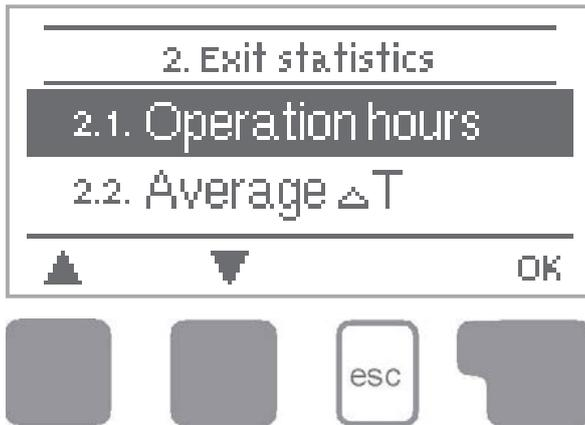
The menu “2. Statistics” is used for function control and long-term monitoring of the system.
