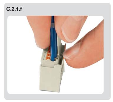
To remove the female connector block from the header, carefully bend the latch on the header.
