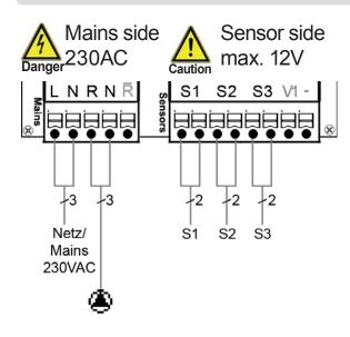
Brief description of switching function: The  $\Delta T$  function sensor 1 > sensor 2 switches the pump at relay R.
