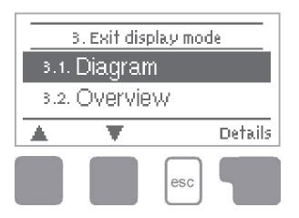
Menu "3. Display mode" is used to define the controller's display for normal operation. This display appears whenever two minutes go by without any key being pressed. The main menu appears again when a key is pressed. The menu is closed by pressing "esc" or selecting "Exit display mode".
