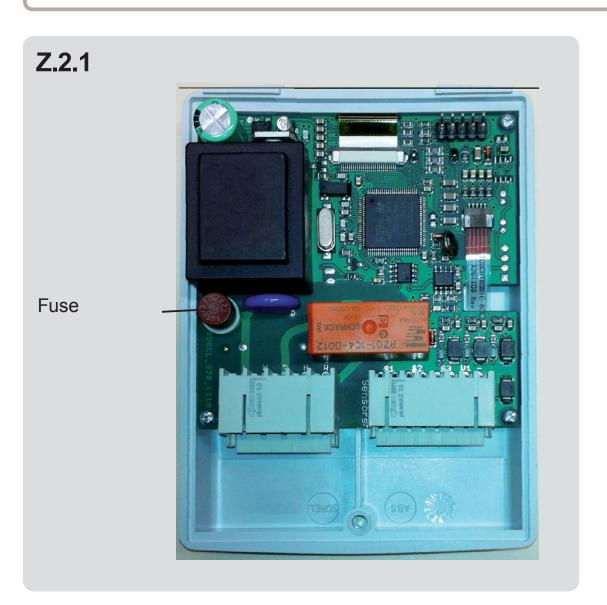
If the mains voltage is switched on and the controller still does not function or display anything, then the internal device fuse may be defective. In that case, open the device as described under C.1, remove the old fuse and check it. Exchange the defective fuse for a new one, locate the external source of the error (e.g. pump) and exchange it. Then first recommission the controller and check the function of the switch outputs in manual mode as described under 4.2.
