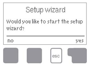
The first time the controller is turned on and after the language and time are set, a query appears as to whether you want to parametrise the controller using the commissioning help or not. The commissioning help can also be terminated or called up again at any time in the special functions menu. The commissioning help guides you through the necessary basic settings in the correct order, and pro-
