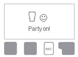
With the party function the storage temperature is heated up once to the reference temperature (Tref off), disregarding the set thermostat times.
