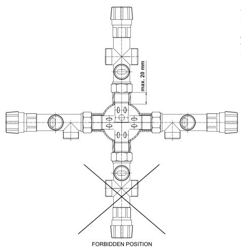
The thermal safety relief valve can be mounted vertically as well as horizontally. In a horizontal position the hot water outlet marked "C" (Fig. 1 and 2) must be facing downwards. The valve must not be installed with its head down!
