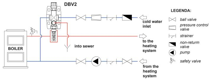
Fig. 3: Piping diagram for DBV2
