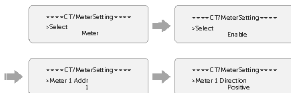
Figure 14-18 Setting meter for the inverter
