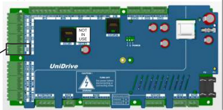
Hauptplatine PCB: UniDrive
